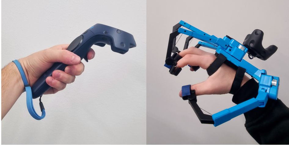
Fig. 2. The two interaction methods used to handle virtual objects. On the left side, the user has the HC (HTC Vive Pro Controller) in his hand, and on the right side, he is using the FG (Senseglove DK1).
